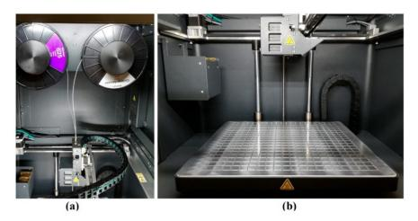
Figure 3. MetalX 3D printer. (a) Material storage chamber and (b) printing chamber.
