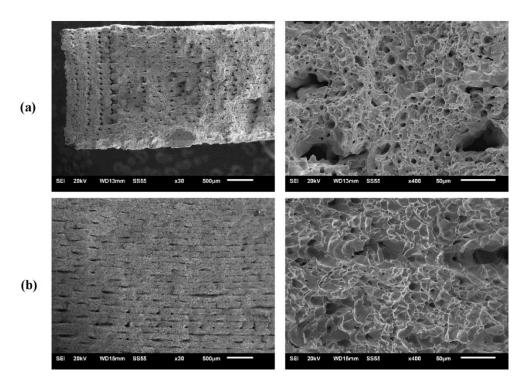
Figure 9. Fracture surface structure of copper MEAM parts. (a) Tensile sample. (b) Charpy sample.
