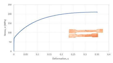
Figure 8. Stress-strain curve of copper Material Extrusion Additive Manufacturing part.
