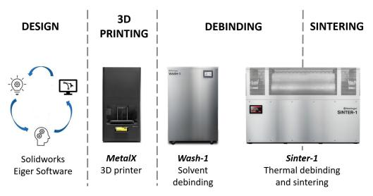
**Figure 2.** Flow chart of the manufacturing process of copper parts with Metal Extrusion Additive Manufacturing technique using the Markforged equipment.
