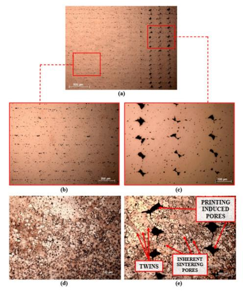
**Figure 7.** Cross section micrographs of sintered copper parts. (a) General view ( $\times$ 50). (b) Interior area with solid infill printing strategy ( $\times$ 200). (c) External perimeter with contouring printing strategy ( $\times$ 200). (d) Microstructure in interior area. (e) Microstructure in external perimeter.
