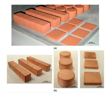
**Figure 5.** Copper parts manufactured by Metal Extrusion Additive Manufacturing. (a) Green parts after printing stage. (b) Final sintered parts.
