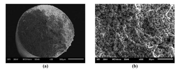
**Figure 1.** SEM micrographs of the copper filament cross section. (a) Details of the inner configuration of filament showing its cylindrical geometry. (b) Details of copper powder morphology and the binder system.
