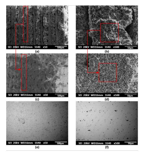
**Figure 6.** SEM images of  $(\mathbf{a},\mathbf{b})$  green part,  $(\mathbf{c},\mathbf{d})$  brown part and  $(\mathbf{e},\mathbf{f})$  sintered final part.  $(\mathbf{a},\mathbf{c},\mathbf{e}) \times 50$ ,  $(\mathbf{b},\mathbf{d},\mathbf{f}) \times 500$ .  $(\mathbf{a}-\mathbf{c})$  Detail of the porosity inherent of the layer-to-layer manufacturing process.  $(\mathbf{b}-\mathbf{d})$  Detail of the porosity inherent of the filament due to the distance between metal particles.
